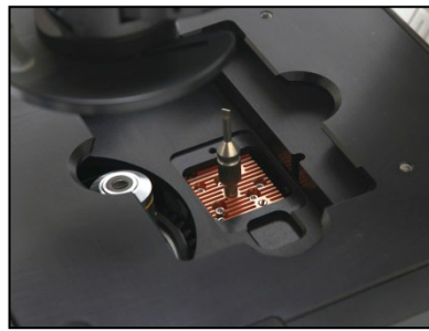
Figure 37 Light cube tool attached to light cube
