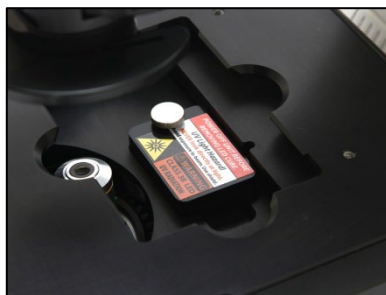
Figure 34 Light Cube Access Cover (under stage)
