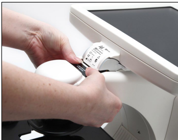
Figure 4 Grasp under support arm with both hands to lift EVOS®
