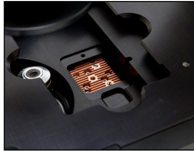
Figure 36 Loosen slotted screws with tool
