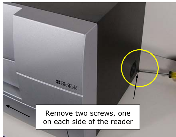
Figure 2: Removing the two side screws.
