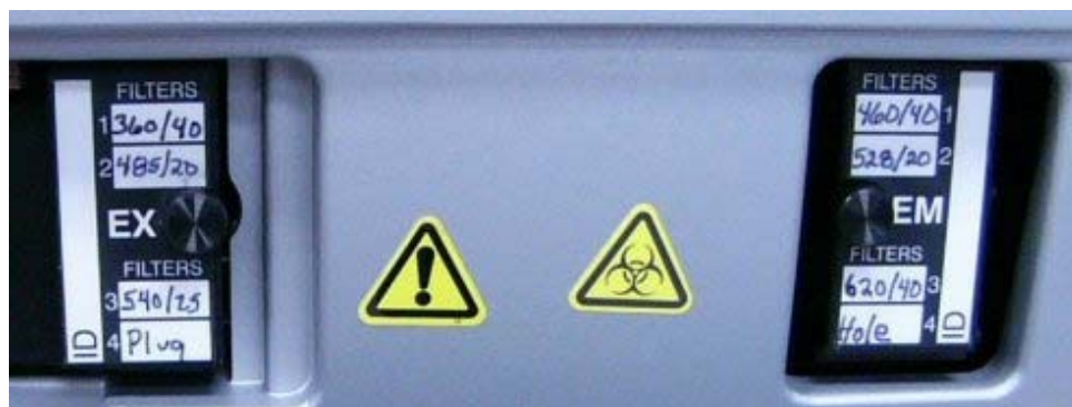
Figure 24: Accessing the Excitation (EX) and Emission (EM) filter wheels
