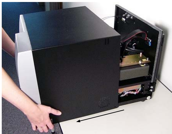
Figure 3: Sliding off the shroud.
