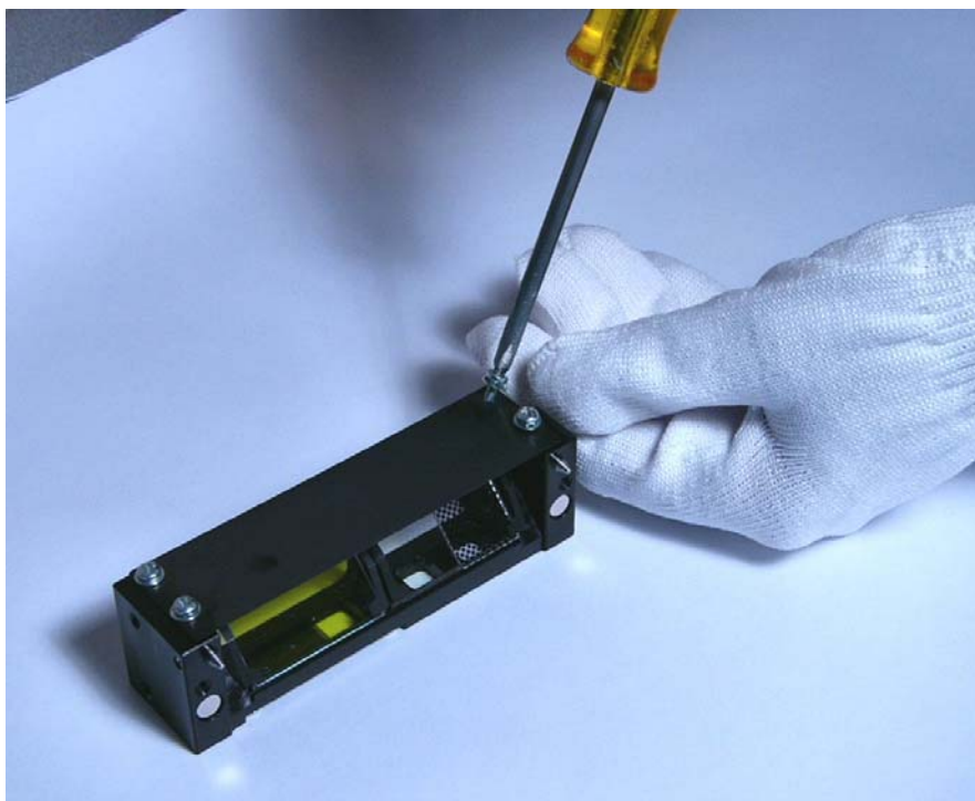
Figure 32: Remove the light shield from the mirror holder
