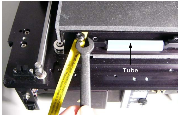
Figure 5: Remove microplate carrier shipping screw and tube.
