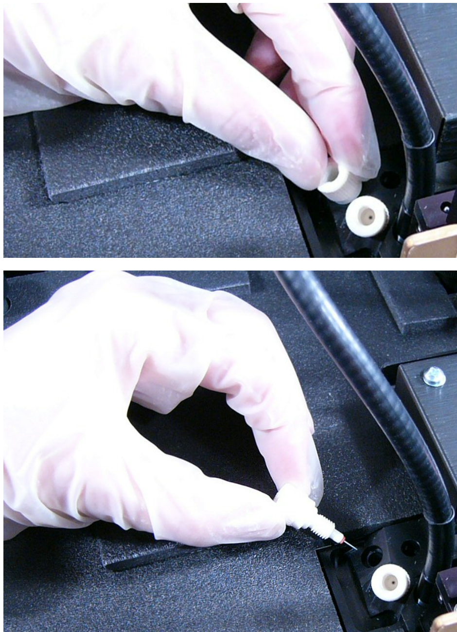
Figure 44: Remove the injector heads
