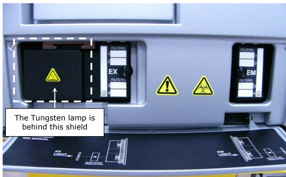
Figure 18: Locating the Tungsten lamp
