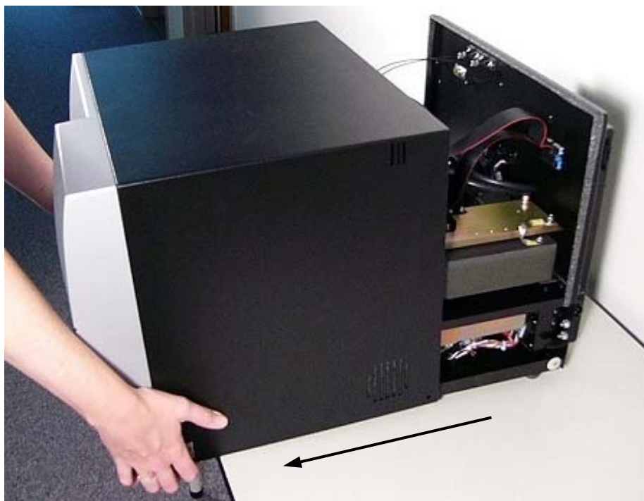
Figure 40: Removing the reader's shroud
