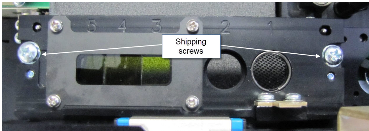
Figure 10: Remove mirror holder shipping screws.
