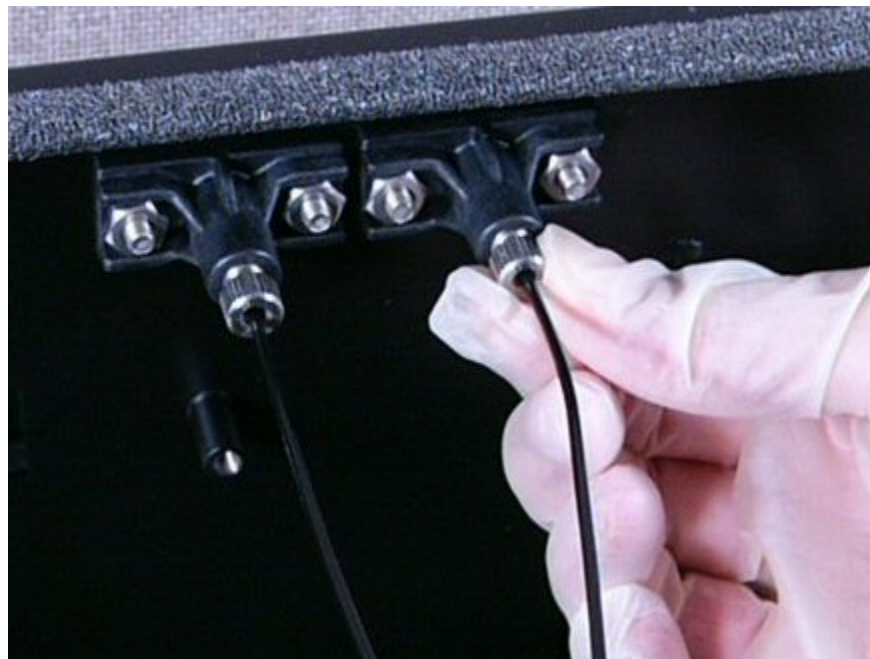
Figure 42: Disconnect the dispense tubes from the back wall
