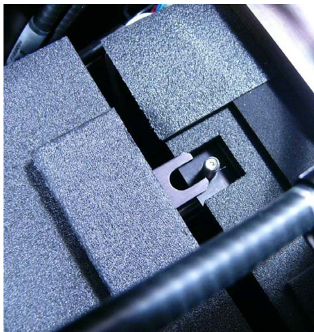
Figure 53: Incubator housing “fork” in the correct position
