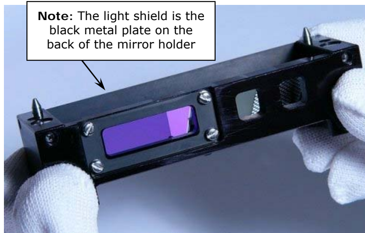
Figure 31: Mirror holder removed from the reader
