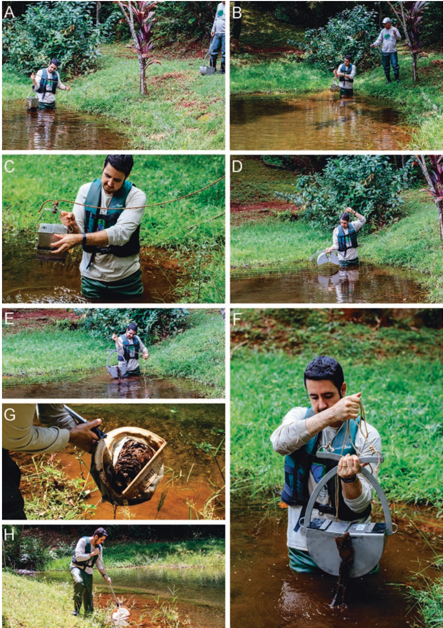
Fig. 20.6 Field sediment sampling using Eckman-Birge dredge (a, b, c), Petersen dredge (d, e, f), and D-net (g, h) at the littoral region of a lentic habitat
