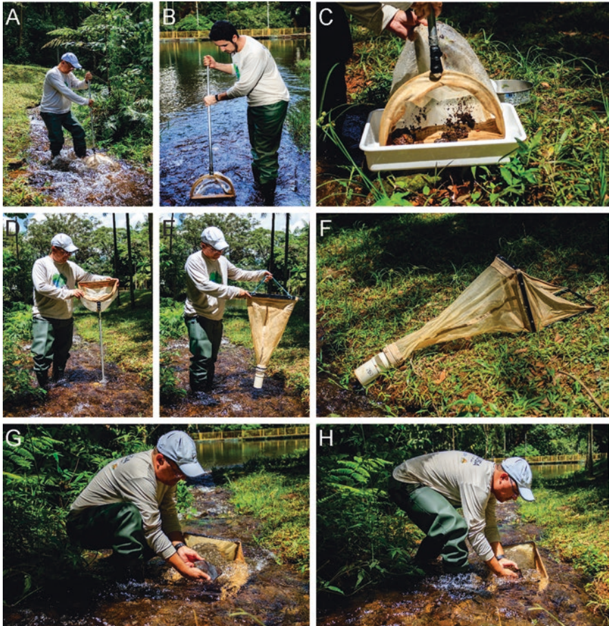
Fig. 20.4 Pictures of field samplings using D-nets (a–d), drift net (e), and Surber sampler (f–h)
