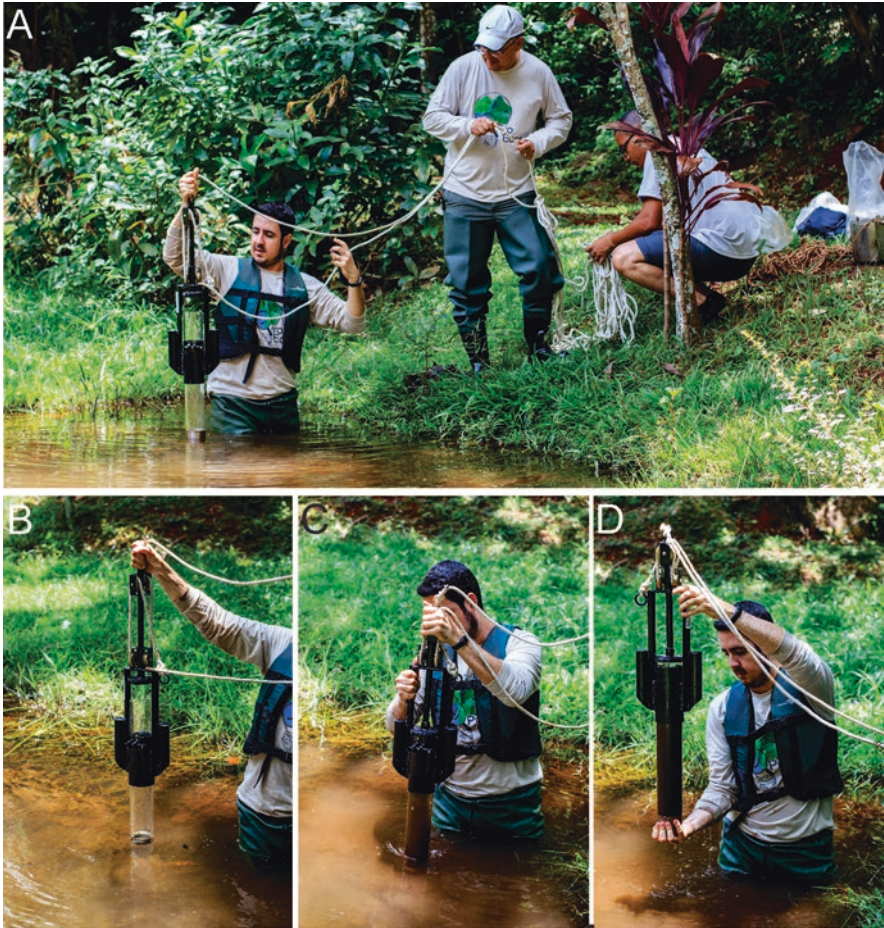
Fig. 20.5 Field sediment sampling using a corer sampler
